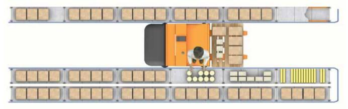
Each model of machine needs its own type of guide rail and a distinct aisle width. The aisle width is defined by the distance between the guide rails and the distance between the load levels.
