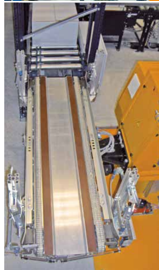
Details of the extraction system that combines forks with belts (EC).
